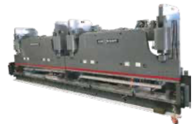
Large Press Break 6.7 Meters Long Up to 1/4" Thk.
