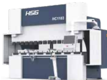
CNC Bending 3 Meters Long Up to 3/8" Thk.
