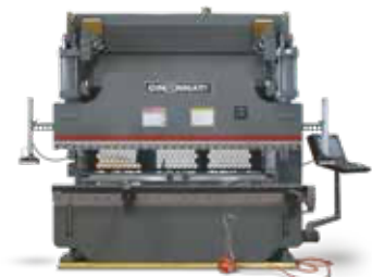
Large Press Break 6 Meters Long Up to 1" Thk.
