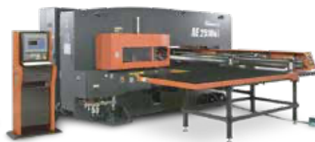
Turret Punch Press 2 Available 30 tons
