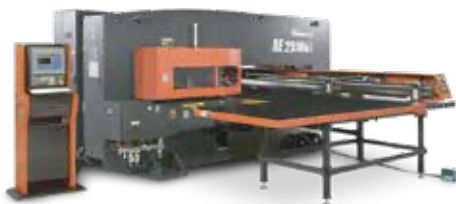
Turret Punch Press 3 Available 50 tons
